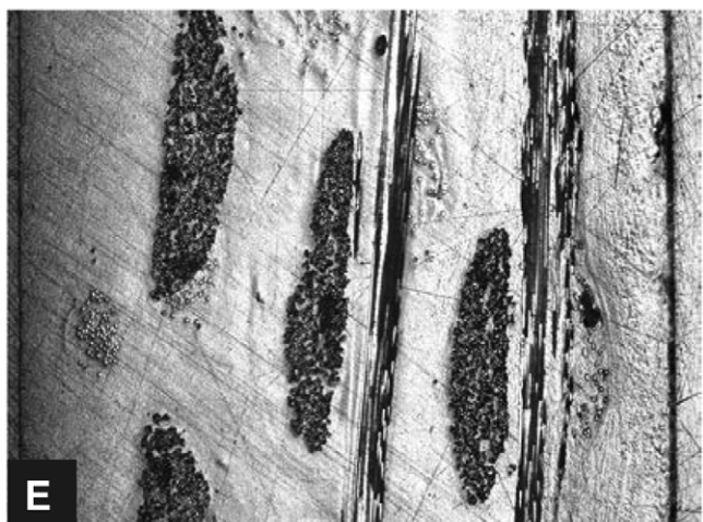
Figure 4. Reflection light microscopy images of APA6/glass fiber composites obtained at magnifications of \times 5 (A, C, and E) and \times 20 (B, D, and F). Composite designations are according to Table I. Each laminate contains five layers of glass fiber fabrics with different densities and weave types corresponding to 20 wt % with respect to ECL.
